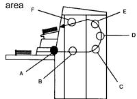
The sensors in the feeder/horizontal transport area are located under the Document Scanning Array, behind the feed/separator rollers, near the reflector strips:
